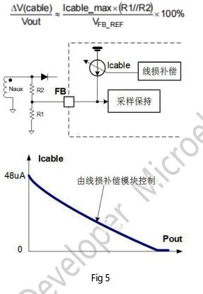
For example,  $R1=2K\Omega$ ,  $R2=16K\Omega$ , The percentage of maximum compensation is given by
